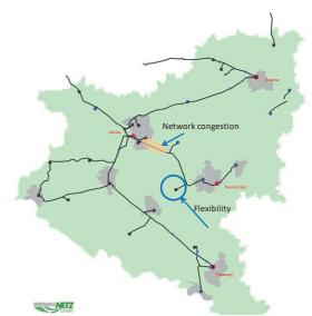
**Figure 6** 110-kV-grid of WEMAG Netz with the location of the flexibility potential
